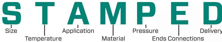
**Size:** Determine the I.D (internal diameter) and O.D (outside diameter) along with the most likely route for the hose installation to calculate the length.
